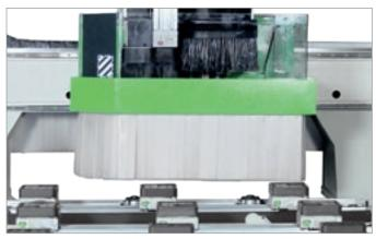
**Side curtain guards** to protect the working unit, which are movable to enable the machine to work at maximum speed in total safety.
