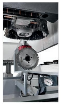
The **Pick-up station** allows a safe tool change on the electrospindle.
